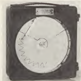
20-11. A recording pressure gauge. (Electric Auto-lite Co.)
